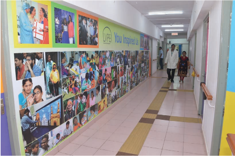
Photographs of the inspiring lives of vision rehabilitation clients adorn the corridor walls, and the floor is modified to include rows of tactile tiles on ground zero, Gullapalli Pratibha Rao building, Kallam Anji Reddy campus, Hyderabad, 2016.
