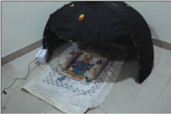
Pediatric perimeter- A device to estimate visual fields in infants (3-6 months of age) Mentor – Dr Premnandhini Satgunam, LVPEI
