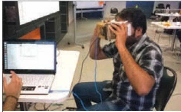
Pupil hacker- A portable pupillometer which checks a patient's response to stimulation by light. Mentor - Dr Anthony Vipin Das, LVPEI
